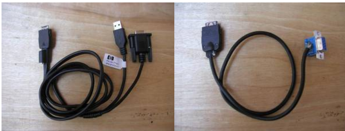
Figure 4 Data cable modification (a) Standard cable (b) Modified cable
