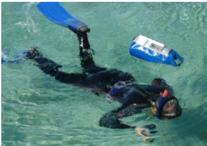
Figure 3: Snorkeller and diver towing the GPS-drybag-float system GPS Photo Transect Manual 3.0
