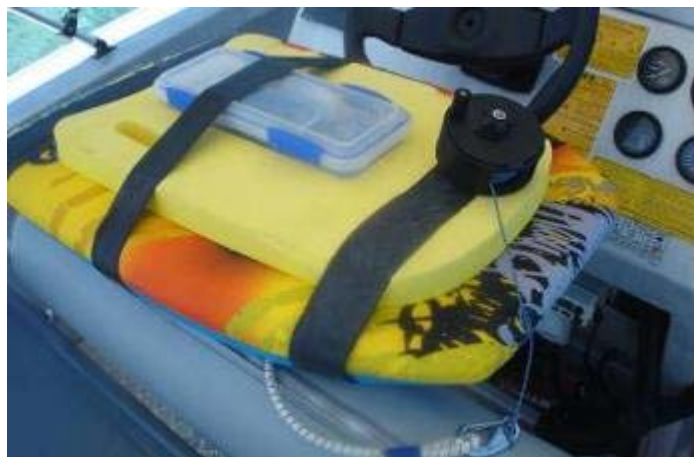
Figure 2: Alternative float set up with GPS place in plastic box within a float and connected to reel (photo: Ray Berkelmans, AIMS)
