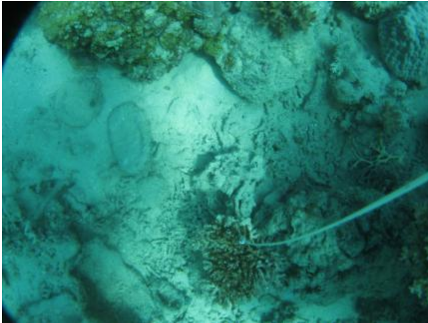
Figure 6: Example photo of benthos, with plump line for set distance from camera to bottom.
