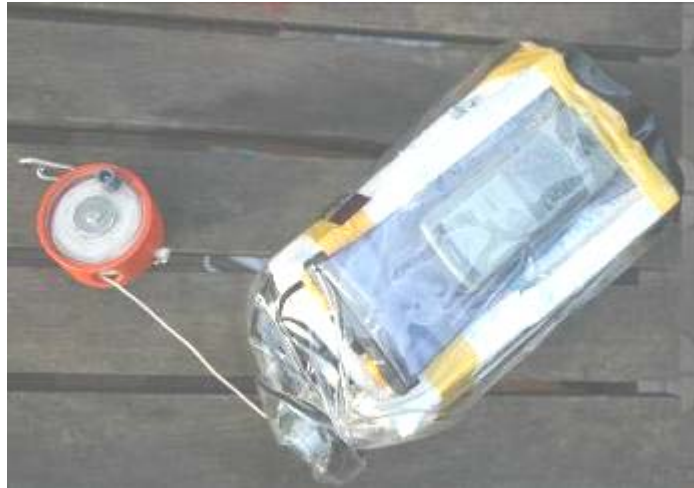
Figure 1: Drybag setup with GPS and Reel.
