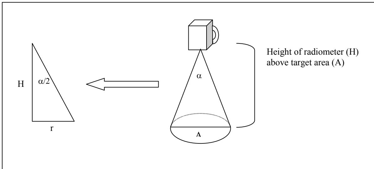
Worked example to establish sample height for a  $1.0\text{m}^2$  target area (A)
