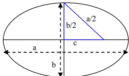
Once the lengths of the major and minor axes ( $a$  and  $b$ ) are known  $c$  can be computed using the pythagorean relation:
