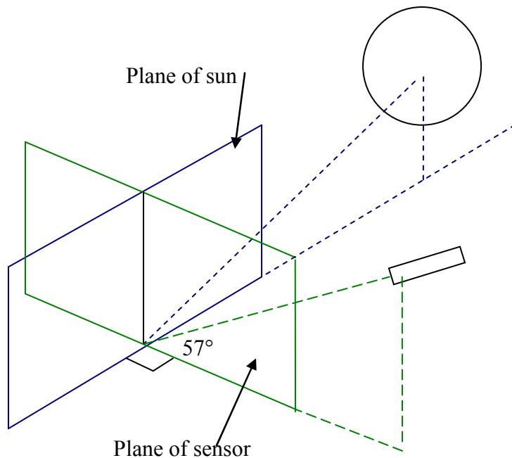
The height at which the spectrometer is held will determine the size of the area sampled as the bare fibre has a  $25^\circ$  FOV. The region will be a circle of approximately 44cm in diameter when held 1m directly above the target (i.e. at nadir). If the sensor is held 1m above the ground, using the CSIRO geometry the sampled region will be an ellipse with minor axis (b) of length 44cm and major axis (a) of 67 cm.
