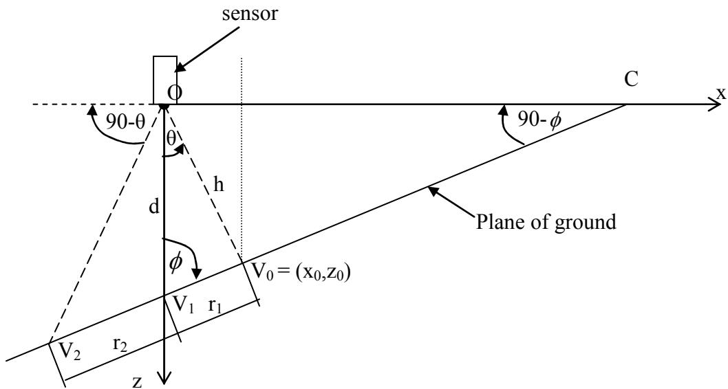
Note that  $\phi$  is half the foreoptic angle and  $\theta$  is the angle between the foreoptic and the horizontal plane of the ground (57 degrees in the CSIRO geometry). From the diagram  $r_1$  is equal to the distance from  $V_0$  to  $V_1$  and  $r_2$  is equal to the distance from  $V_1$  to  $V_2$ . These distances can be computed using the euclidean distance rule:
